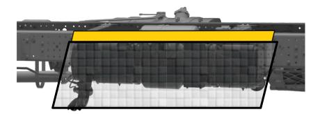
Clearance of Min 50mm to be maintained above the ATS area
