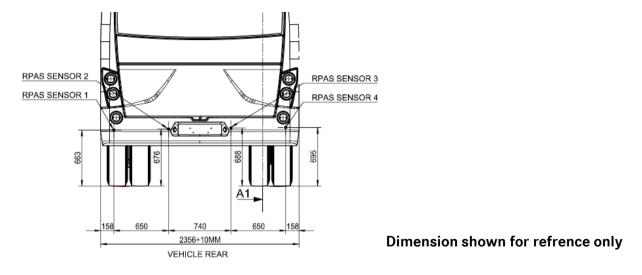
2. Install the RPAS sensor assembly (A) and Bezel (B) on the rear dome of Bus body using snap fit.
