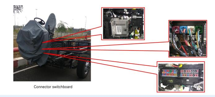
The cabin Fuse box & Relay mounting bracket should be given by Bus body builder and should be enclosed to avoid damage.
