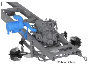
The air filter assembly must not be repositioned.
