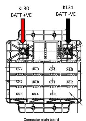
KL30: (+VE) X6.1 – CHASSIS INTERCONNECTOR X6.9 – CHASSIS INTERCONNECTOR
