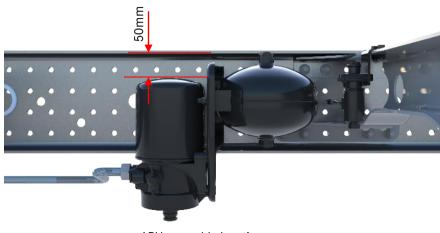
APU assembly location Min. distance between body = 30mm
