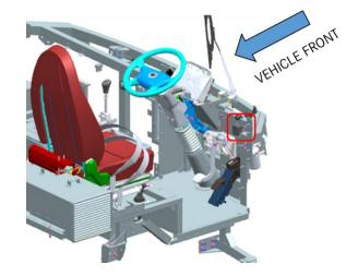
Install the RPAS Buzzer (6) to mount on driver comportment with M6 Pan head Screws (4) using 5 size Allen Key. Set the torque to 7.8 ± 0.6 Nm.
