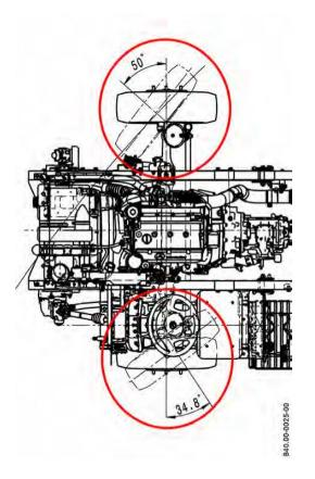
The wheelhouses must make possible the free movement of the wheels, i.e., the wheels must not have their movement prevented when they are fully turned or during the flexure of the suspension system. Foresee clearances for the steering system movements.
