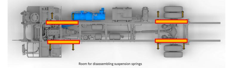
Check the possibility of disassembling the front and rear suspension springs, as shown in the figure.
