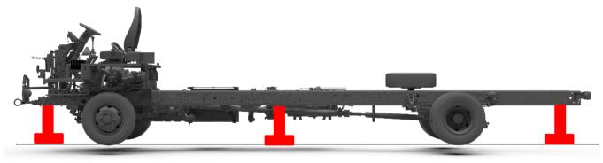
Chassis alignment and leveling
