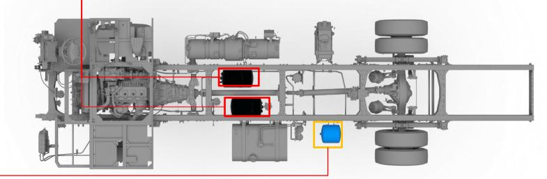
Position of Air tank on OF917 4250WB chassis
