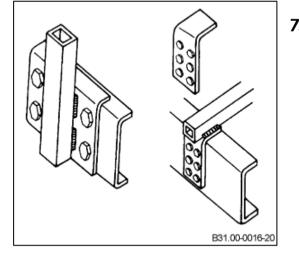
Body fastening by means of corner plates
