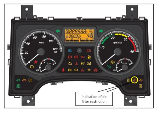
Air filter restriction indication on instrument cluster
