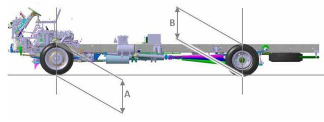
Chassis height A Frame height near front axle, to ground level B Frame height near rear axle, to ground level
