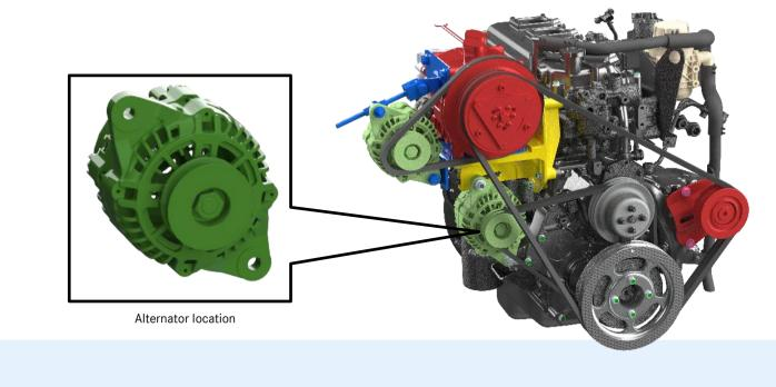
Alternators cannot be switched on before being duly connected to the vehicle's batteries, since this causes an electrical surge that damages electronic modules and voids the electronic module and alternator warranty, as a result.
