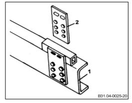
Body fastening by means of corner plates
