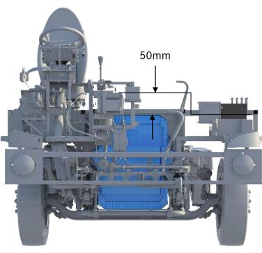
Min. gap between cooling system
