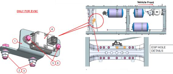
The ESC Module is Fitted in the Middle of the chassis and is calibrated from the factory. Tampering, removing, repositioning the ESC
