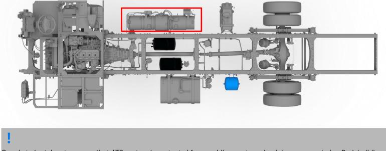
Care is to be taken to ensure that ATS system is protected from welding spots and paint overspray during Bodybuilding.
